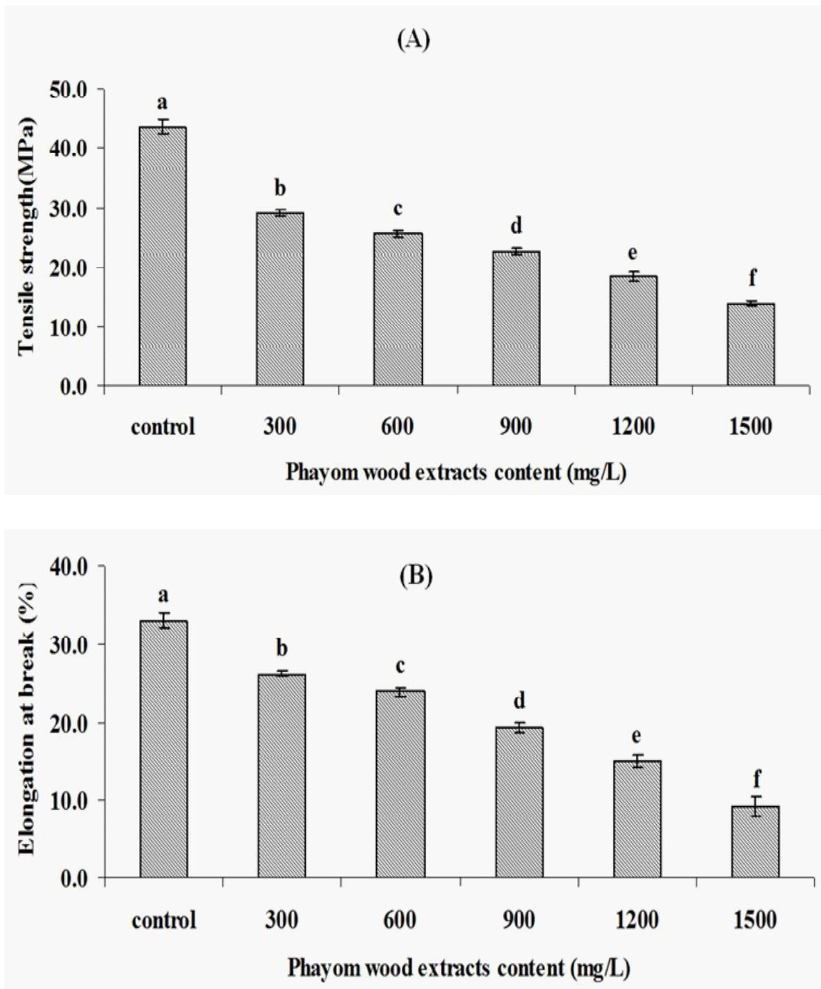
**Figure 2.** Tensile strength (A) and elongation at break (B) of HPMC films as a function of phayom wood extract concentration (error bars are standard error of the mean of five measurements from three separate films). Different letters indicate significantly different groups determined by Duncan's test ( $p < 0.05$ ).
