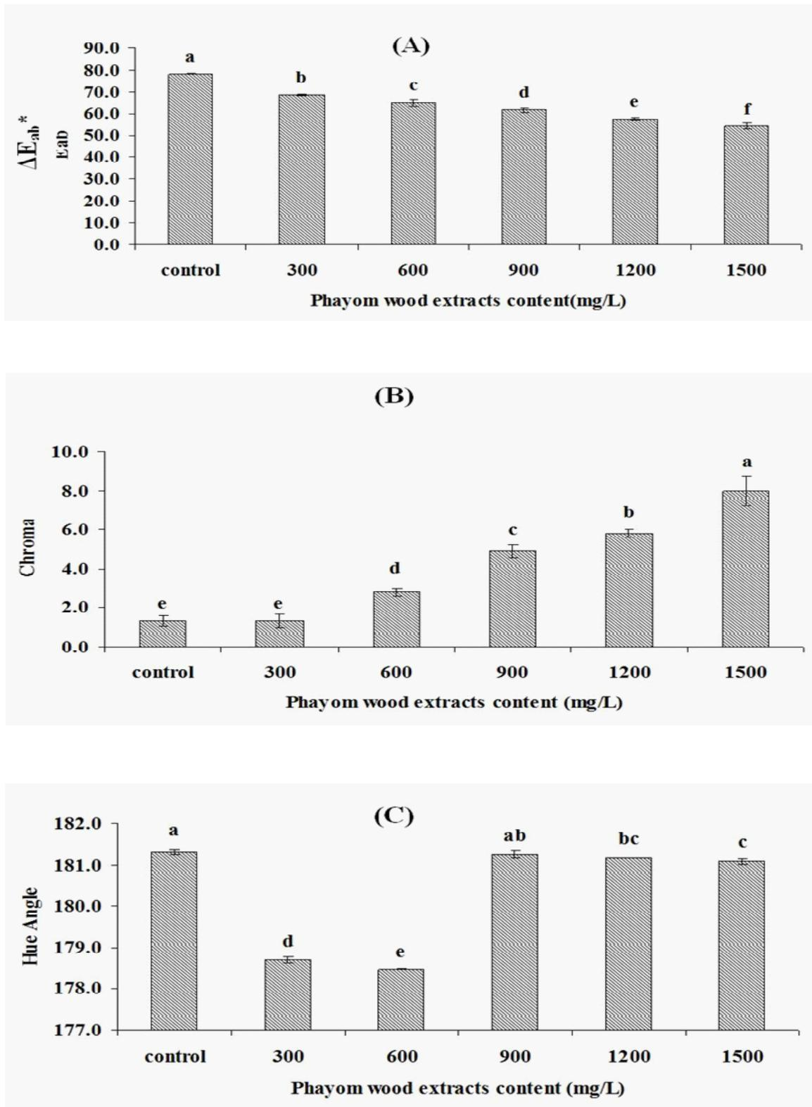
**Figure 5.**  $\Delta E_{ab}^*$  (A), chroma (B) and hue angle (C) of edible HPMC films as a function of phayom wood extract concentration (error bars are standard error of the mean of five measurements from three separate films). Different letters indicate significantly different groups determined by Duncan's test ( $p < 0.05$ ).
