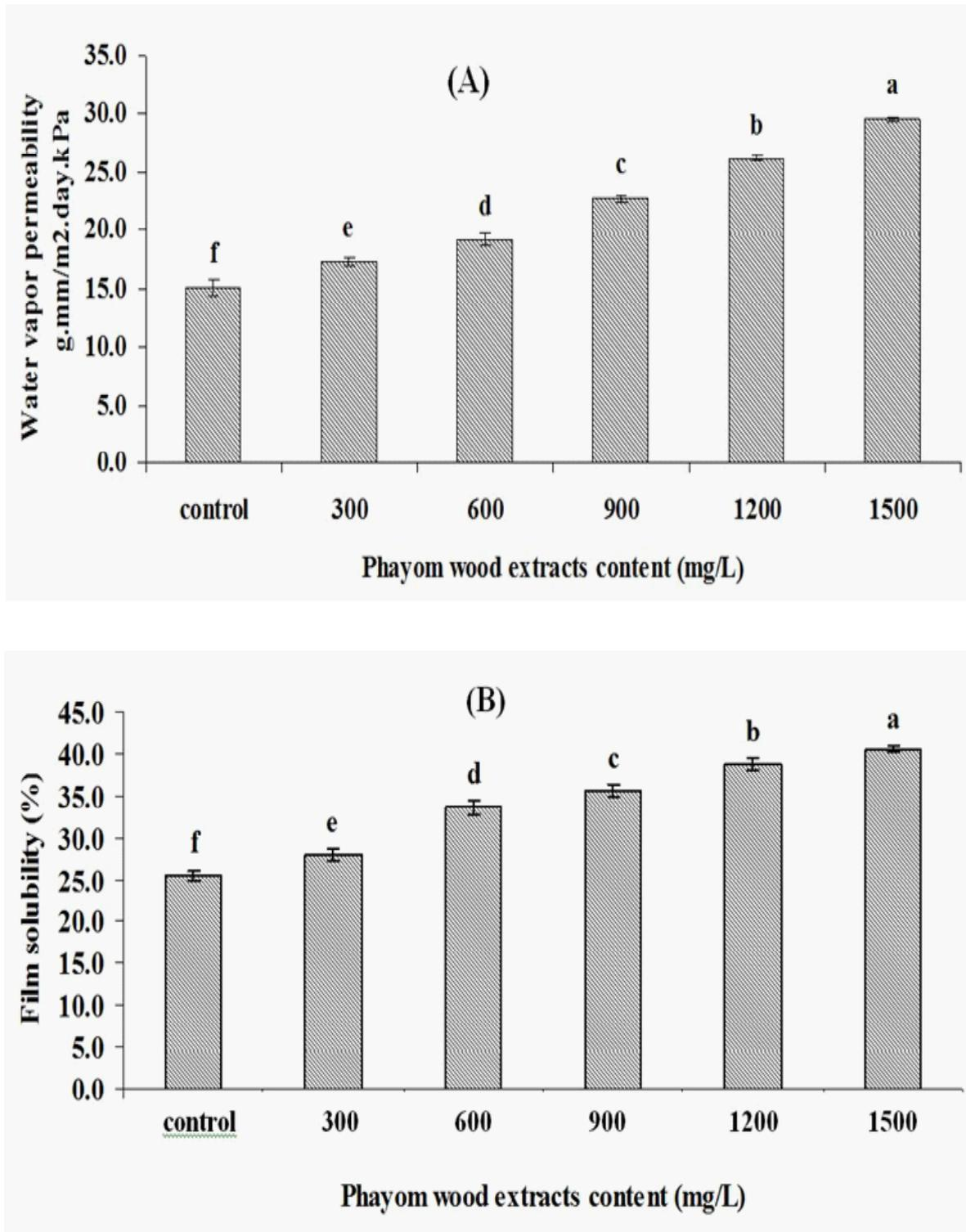
**Figure 3.** Water vapor permeability (A) and film solubility (B) of edible HPMC films as a function of phayom wood extract concentration (error bars are standard error of the mean of five measurements from three separate films). Different letters indicate significantly different groups determined by Duncan's test ( $p < 0.05$ ).
