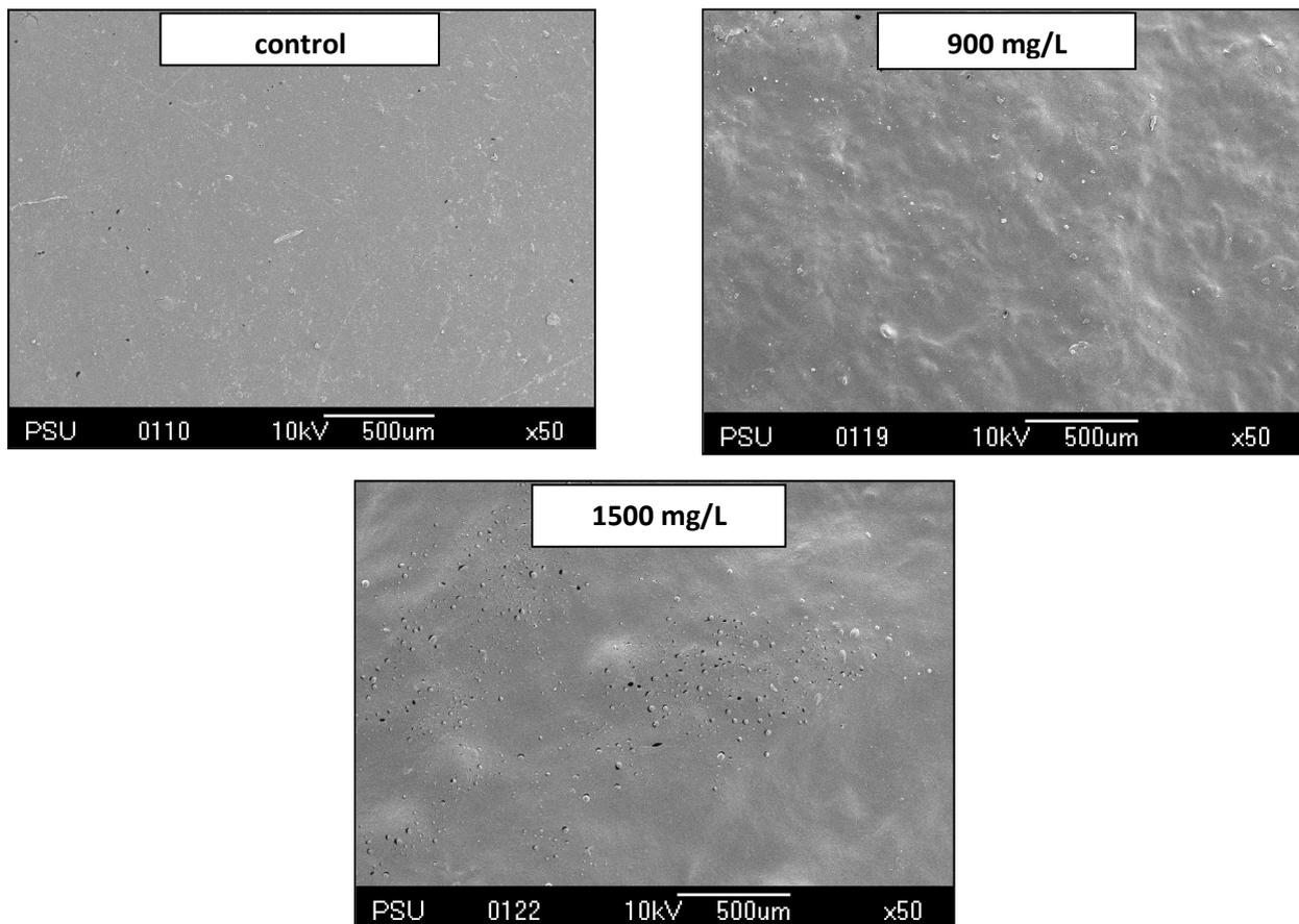
**Figure 7.** Scanning electron micrograph of edible HPMC films containing 900 mg/L and 1500 mg/L phayom wood extract.
