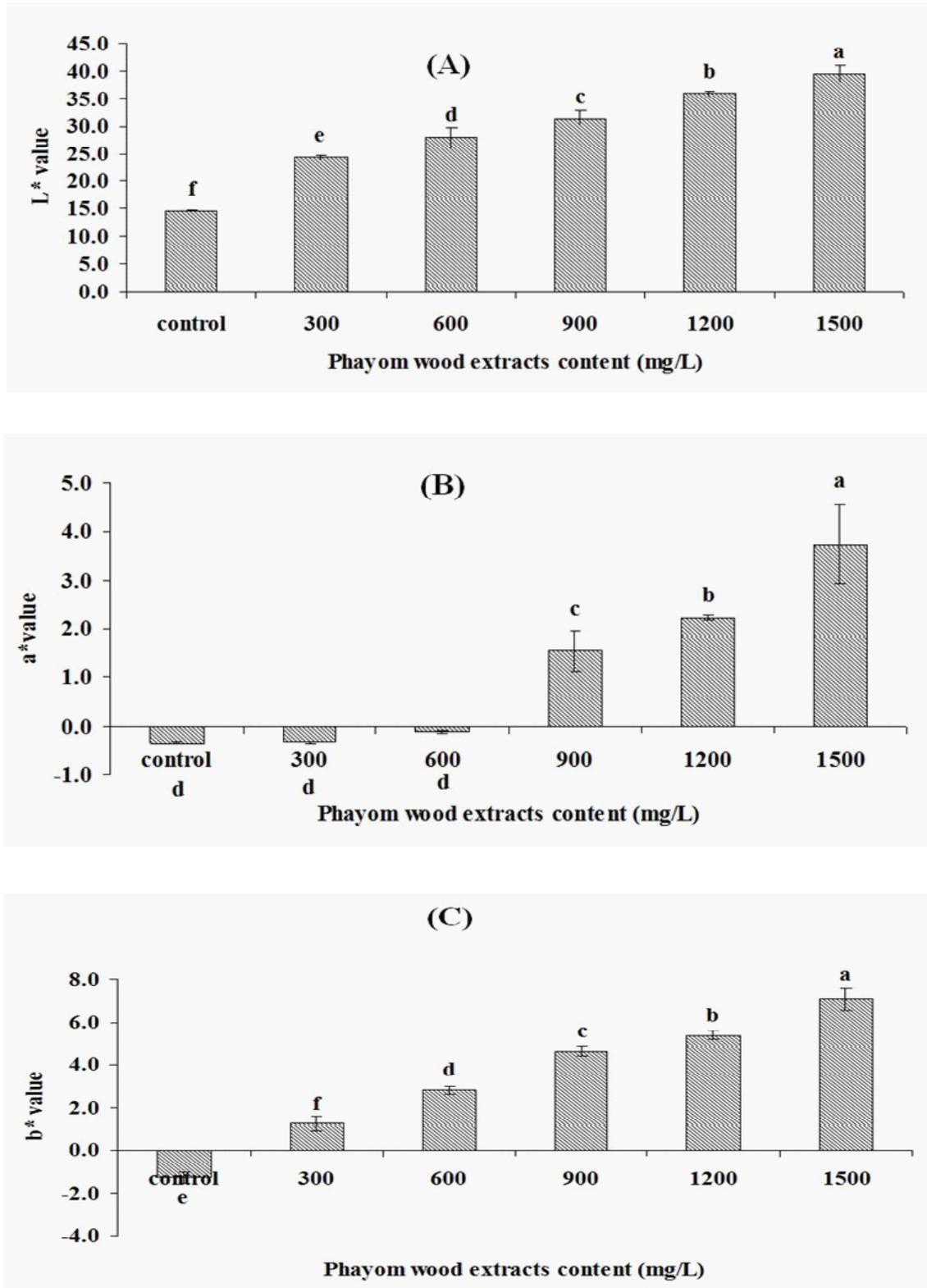
**Figure 4.** L\* (A), a\* (B) and b\* (B) values of edible HPMC films as a function of phayom wood extract concentration (error bars are standard error of the mean of five measurements from three separate films). Different letters indicate significantly different groups determined by Duncan's test ( $p < 0.05$ ).
