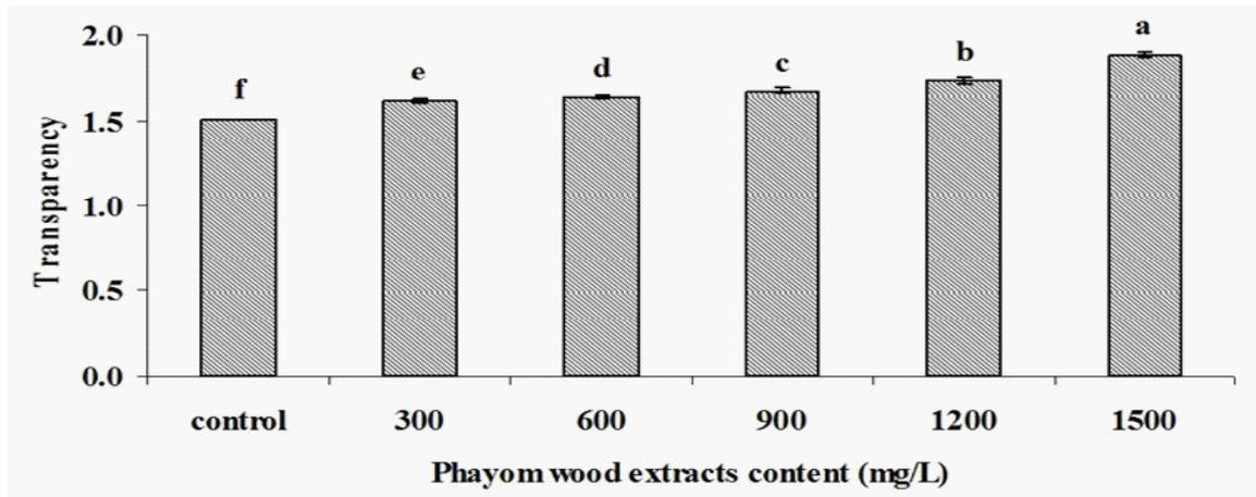
**Figure 6.** Transparency of edible HPMC films as a function of phayom wood extract concentration (error bars are standard error of the mean of five measurements from three separate films). Different letters indicate significantly different groups determined by Duncan's test ( $p < 0.05$ ).
